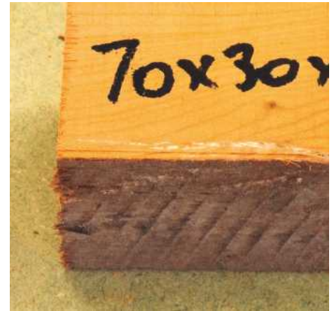
▲ Pic.3 One of the problems with yew is the appearance of faults like this. Silver shake appears naturally in the timber and is very difficult to fix, so is best turned away
